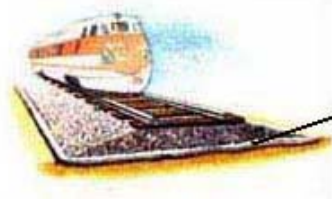
Gravel separated from soil by sheets of Urim Fabrics to prevent sinking and dispersion.
